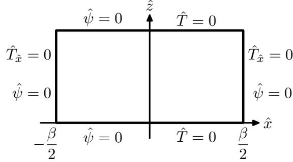
Figure 4: Convection cell with with impermeable boundaries, fixed temperature at the top and bottom and insulating side boundaries.
