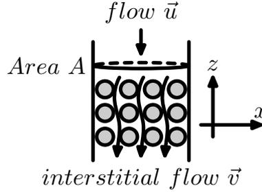
Figure 1: The two rates of flow; the total flow  $\vec{u}$  and the interstitial flow  $\vec{v}$
