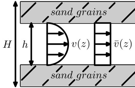
Figure 2: Flow between the interstices of the sand grains as 2-d flow between plates where  $h$  is the average distance between interstices,  $H$  is the interstitial width plus the width of a sand grain,  $v(z)$  is the fluid flow between the interstices and  $\bar{v}(z)$  is the average flow. In this case  $\phi = \frac{h}{H}$ .
